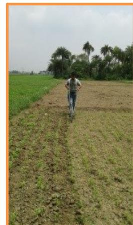
**Photo 2. Operation of SWJW in line sown jute crop**
